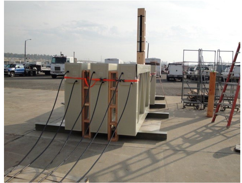
Prototype Ice Harbor Spillway Detection Antennas (2016)
